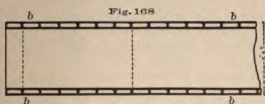
WATER-COOLED FLUE OF SHEET-LEAD.
